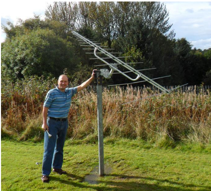
Fig. 5: How to install SAT-rotor for pseudo parallactic mount with tracking in local hour angle only at fixed declination. Depending on mounting method the command for hour angle needs to be changed from ha to -ha.
