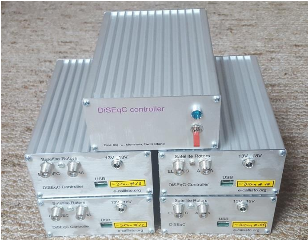
Fig. 1: Final product backside with connectors and front side with LED and switch
