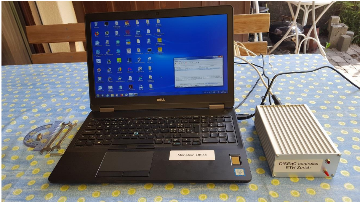
Fig. 8: Control PC and rotor controller box. A Python script is called every 5 minutes and commands the rotor to the actual Sun position. The system can also be used to track satellites, e.g. IRIDIUM.
