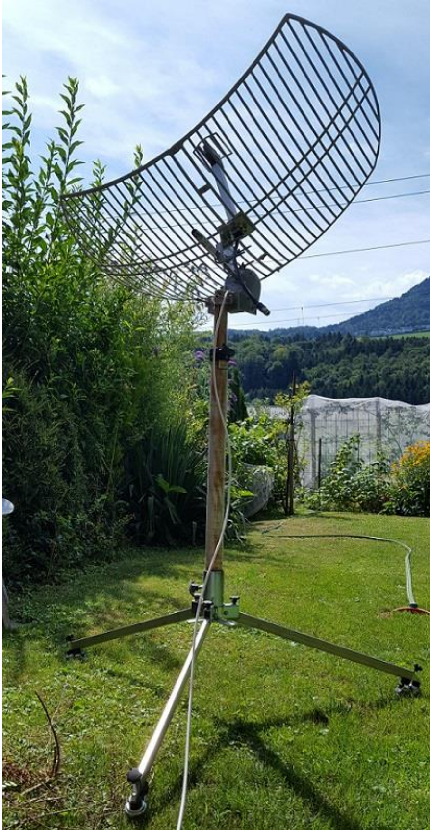
Fig. 9: S-band antenna with Sat-rotor on a tripod tracking the Sun.
